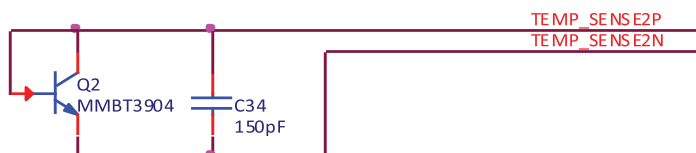
Figure 8.5. NPN Temperature Sensor Circuit
