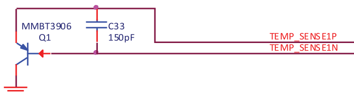
Figure 8.4. PNP Temperature Sensor Circuit
